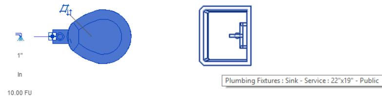
**TARGET: PLUMBING FIXTURE – SOURCE NOT REQUIRED (I.E. WASTE, FOR A VARIETY OF REASONS)**
