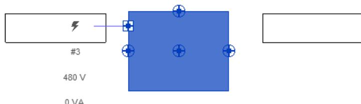
TARGET/SOURCE – TRANSFORMER (TARGET FOR 480/277V PANEL, SOURCE FOR 120/208V PANEL)
