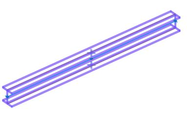
A small number of compound beams do not interfere with the general performance of the project. However, when going to a higher number of compound beams – like hundred(s) and beyond – the impact can be significant. Not only that the number of objects increases exponentially (1:7 in this example), but also because the joint (the intelligence behind the compound) performs additional calculations behind the scene.
