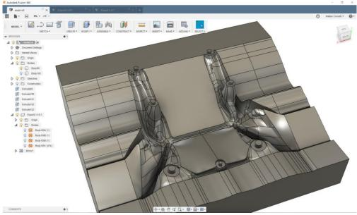
The mold is ready also for machining in the manufacturing environment:
