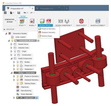
After that, we can hide the Obstacles, so I can apply the design conditions to the Preserve Geometry, starting from the fixed constraints we apply to the four fixings.
