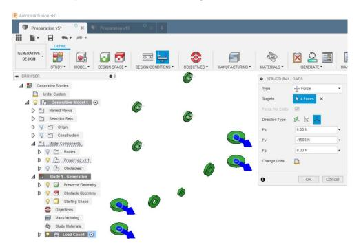
After that, we clone the Load Case 1, so I don't need to reapply the fixed constraints to the fixings.
