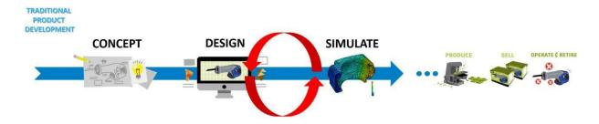
With Autodesk Generative Design, engineers and designers are able to obtain a design space of hypothetical solution based on stating inputs and needs and add those synthetic suggestion to their experience for creating new shape, already optimized and ready for final VALIDATION and FEM analysis.
