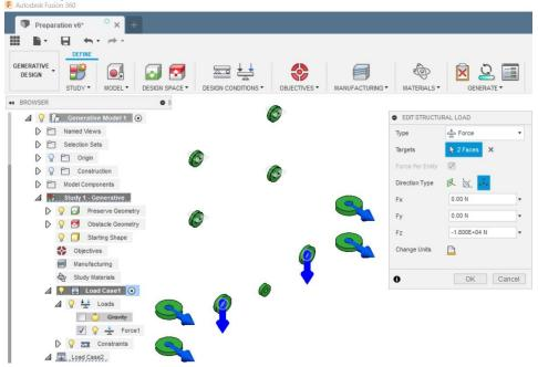
We repeat the step above, cloning the previous load case, editing the Force and applying a force of 500 N in the negative Y direction to the face as in the image below.
