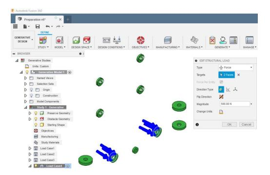
After having defined the Load Cases, we specify the objectives for our results, that, as I wrote above, is mainly to reduce the mass of the existing design, using a Safety Factor of 5.
