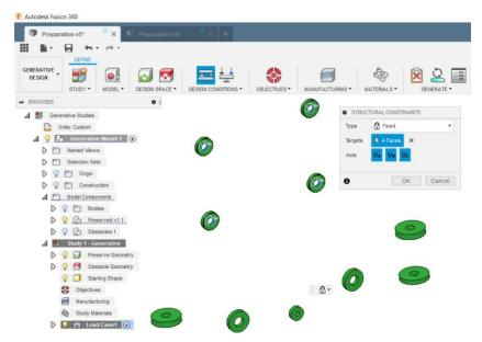
Then, we apply a load of 1500 N in the negative Y direction to the four faces in the image below.
