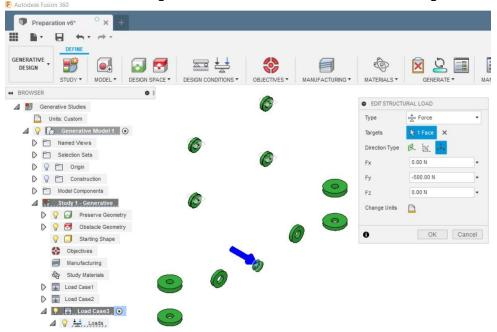
Finally, repeating the same steps, we apply the last force of 500 N perpendicularly to the two faces as in the image below.
