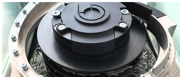
FIGURE 8: TOOLING FOR FEEDING SYSTEM (SOURCE: HOFMANN & STIRNER GMBH WEBSITE).
