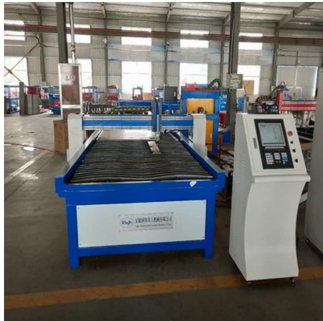
Figure 1: CNC cutting machines typically come with a computer controller loaded with nesting software. Image credit: Rbqly Machines
