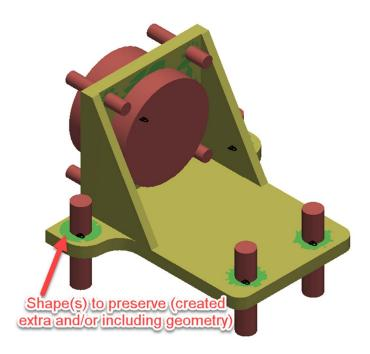
The *Obstacle Geometry* type is geometry which you want AGD to build the optimized design around. These are also known as obstacles. I have created obstacles in the screenshot below so that the holes are not filled within the final design. The bodies assigned to this type will inherit a red color.
