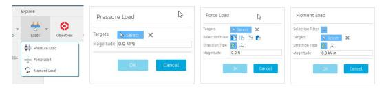
There are 3 different types of Loads to assign within Autodesk Generative Design. A *Pressure Load*, a *Force Load* and a *Moment Load*.
