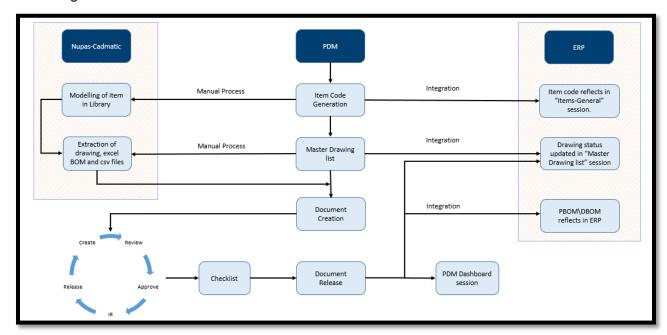
The Master drawing list maintained in the Vault provides the project wise list of drawings to be prepared by design. It also as the provision to maintain the planned scheduled release date against each drawing helps designers to track their priorities.
