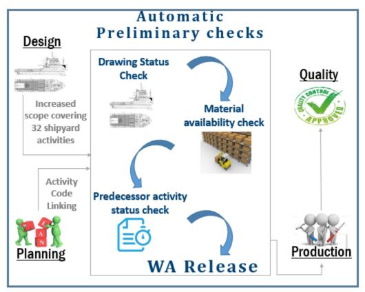
Each activity progress is being monitored and tracked by the Work authorisation closure status and real time dashboards developed for ready reference. WA release status is pushed to PDM vault, which helps design team to know the drawings which are in the production line. This input also enables design to take any decision if there is need of modification in the drawing.
