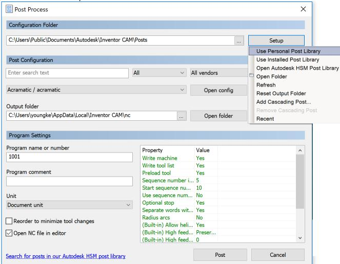
m. Use the post processor for your machine and generate the NC code.
