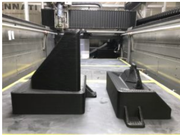
Heated bed on a Cincinnati Incorporated BAAM printer. www.e-ci.com
