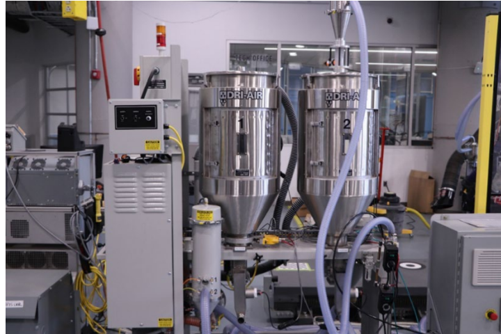
A Dry-Air pellet drying and feeding system
