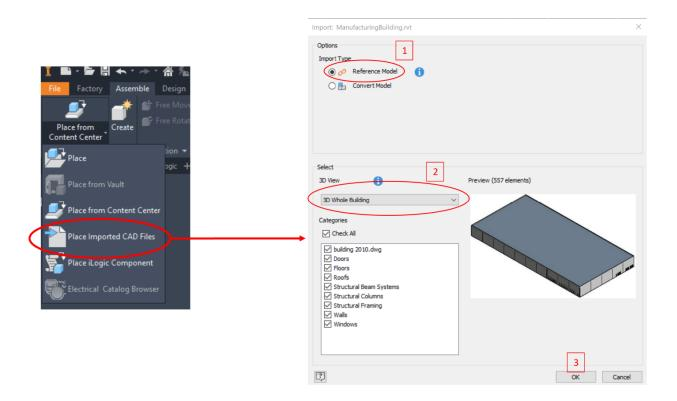
3. The Revit model is inserted "Grounded at Origin" to make sure that the coordinates of the Revit project match the coordinates in Inventor.
