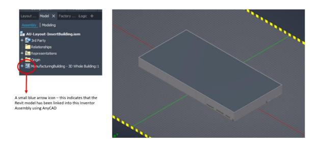
4. Making a change in Revit model also updates the Revit reference model in Inventor. Once changes are saved in Revit and when you switch back to Inventor, you will see the "Orange" lightining symbol next to Revit file name in Inventor browser. Upon clicking the local update button the Revit model inside Inventor also updates to reflect the change made in Revit
