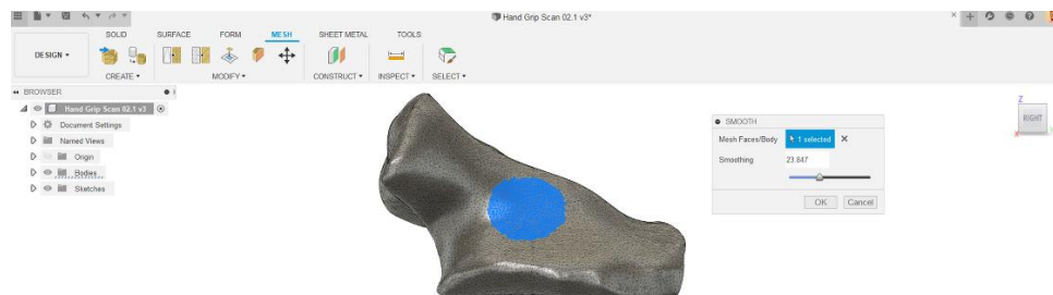
Figure 14: Reverse Engineering with Scan Data – Example Courtesy of PrintCity
