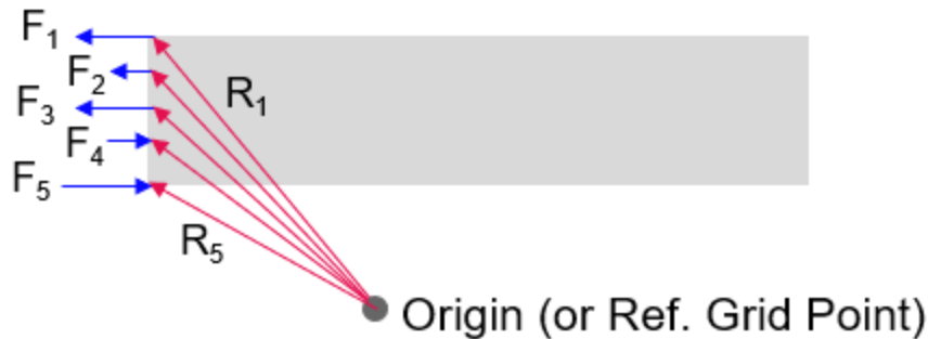
Figure 74 - How the moment reaction is calculated, where M_i is the moment reaction (if it exists) at each node 1 through i .
