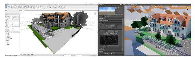
As a first step after importing the rough house and room layout from Autodesk Revit we want to make sure the room has enough natural light and conducted a light study with different times of the day leveraging VRED's procedural skylight environment which allows to simulate different sunlight situations considering location and time.
