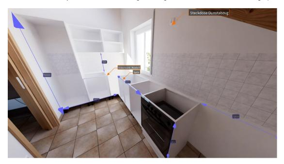
It is worth to mention that VRED comes with an Asset Manager to store the individual kitchen elements in a re-usable library or work with Smart References (aka. Assemblies in CAD). That means, no matter where the basic element is placed in the scene it is possible to work further on an assembly level, update or replace Reference with new CAD data in your main scene.
