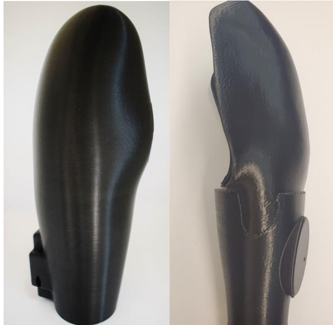
Figure 35: Trans-humeral socket comparison between optimized and original workflow.
