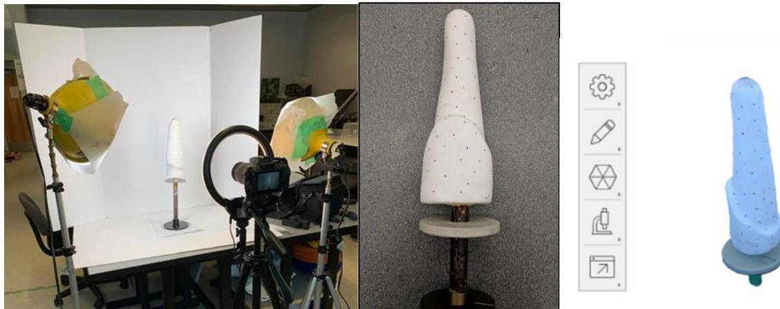
Figure 7: Taking images of the limb positive with a digital camera (left). Using photogrammetry in Autodesk ReCap Pro to generate a digital model of the limb positive (right).
