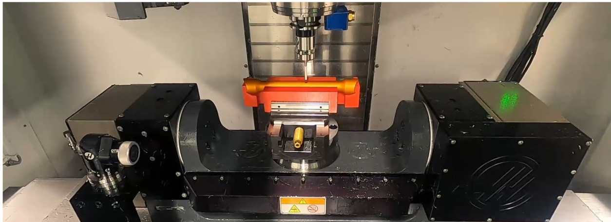
Figure 17 - Part Setup Probing on a CNC Machine Tool
