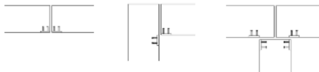
Connection with Anchor Plates
