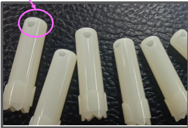
Hole due to Air trap
