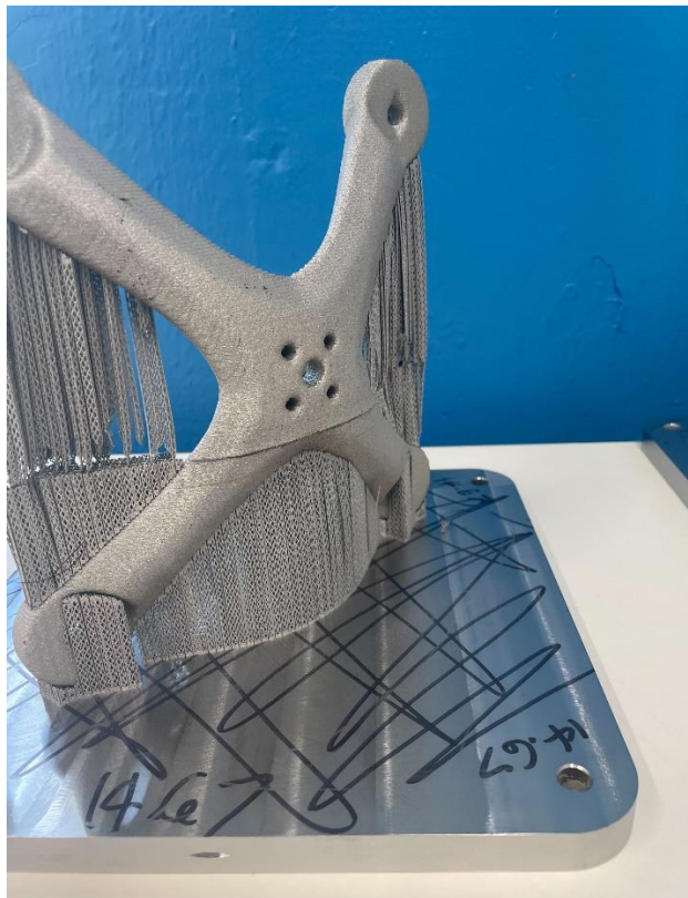
Figure 2 - A failed LPBF print
