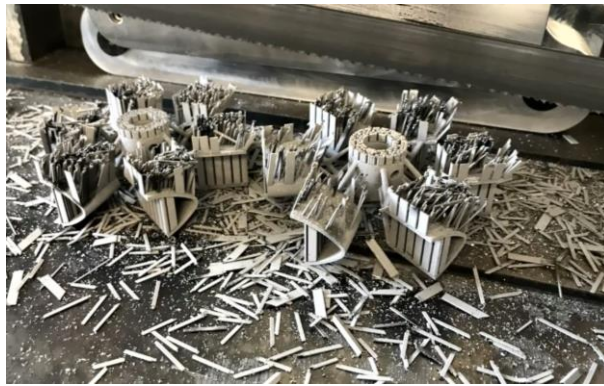
Figure 6 - Support structures removed from a LPBF print
