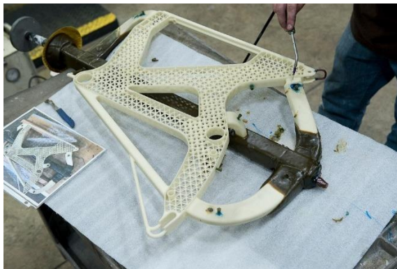
Figure 11 - Polymer print prior to casting
