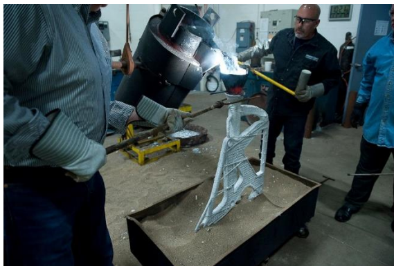
Figure 12 - Casting the metal part
