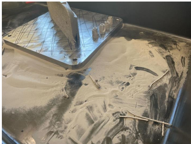
Figure 4 - Excess powder from a LPBF print
