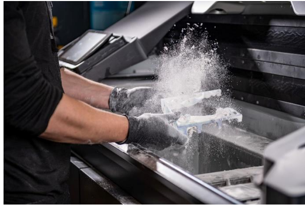
Figure 3 - Removing excess powder from a polymer print
