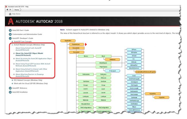
To give you an idea of what an object model looks like, you'll have to go to AutoCAD's Help System. Navigate to the ActiveX concepts in the AutoLISP Developer Guide as shown above to view AutoCAD's Object Model. The links here tell you a lot about how to interact with the ActiveX Object Model using AutoLISP.
