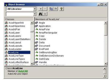
The Visual Basic editor opens the Object Browser with it set to display the AutoCAD Object Model library. Using this object browser won't help any more than using the ActiveX Reference, it's just another way to access the same information.
