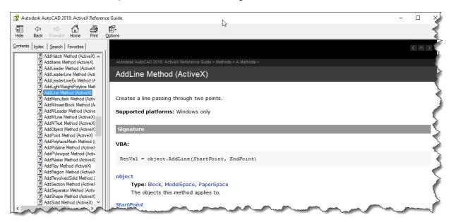
From the help for the *AddLine* method, you can see that Visual Basic requires two arguments. In addition, the *Object* lists several possibilities. The Modelspace collection, Paperspace collection and a Block object. That means that a Line needs to be in either Paperspace, Modelspace or part of a Block definition. In this case, we'll be adding it to the Modelspace collection. What this means
