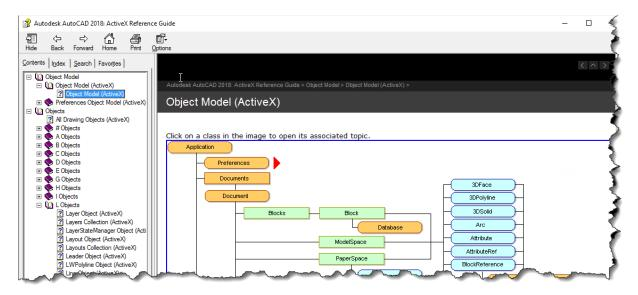
When you get to the Object Model in this version of Help, clicking on any of the items in the Object Model will display information for that item. You'll also notice by looking at the object model that there are rectangular shapes with square corners and rectangular shapes with rounded corners. Looking at the legend, you can see that those with square corners are a *Collection* and those with rounded corners are an *Object*.
