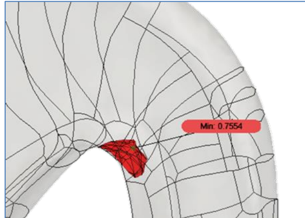
Figure 31 - Load Case 2 (45°) volume with SF \leq 1 [von Mises stress vs. yield strength]
