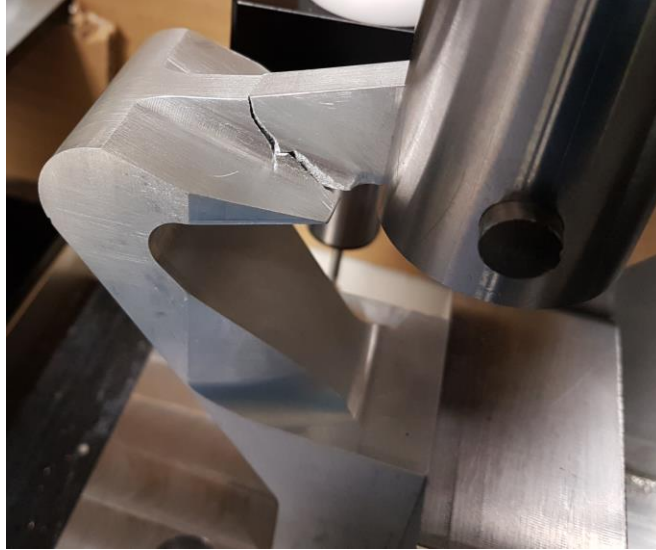
Figure 44 - Failure location of machined bracket
