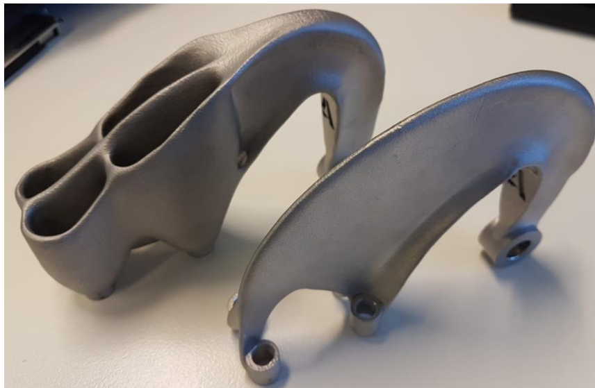
Figure 35 - Generative Design AM Brackets (display models with logo)
