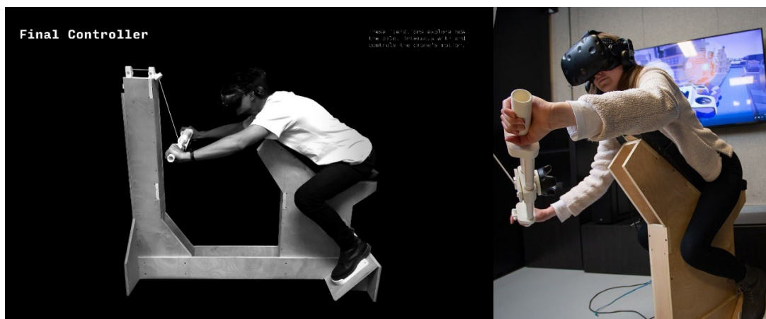
Matt Whitby's buck with sensors to fly a virtual passenger drone.
