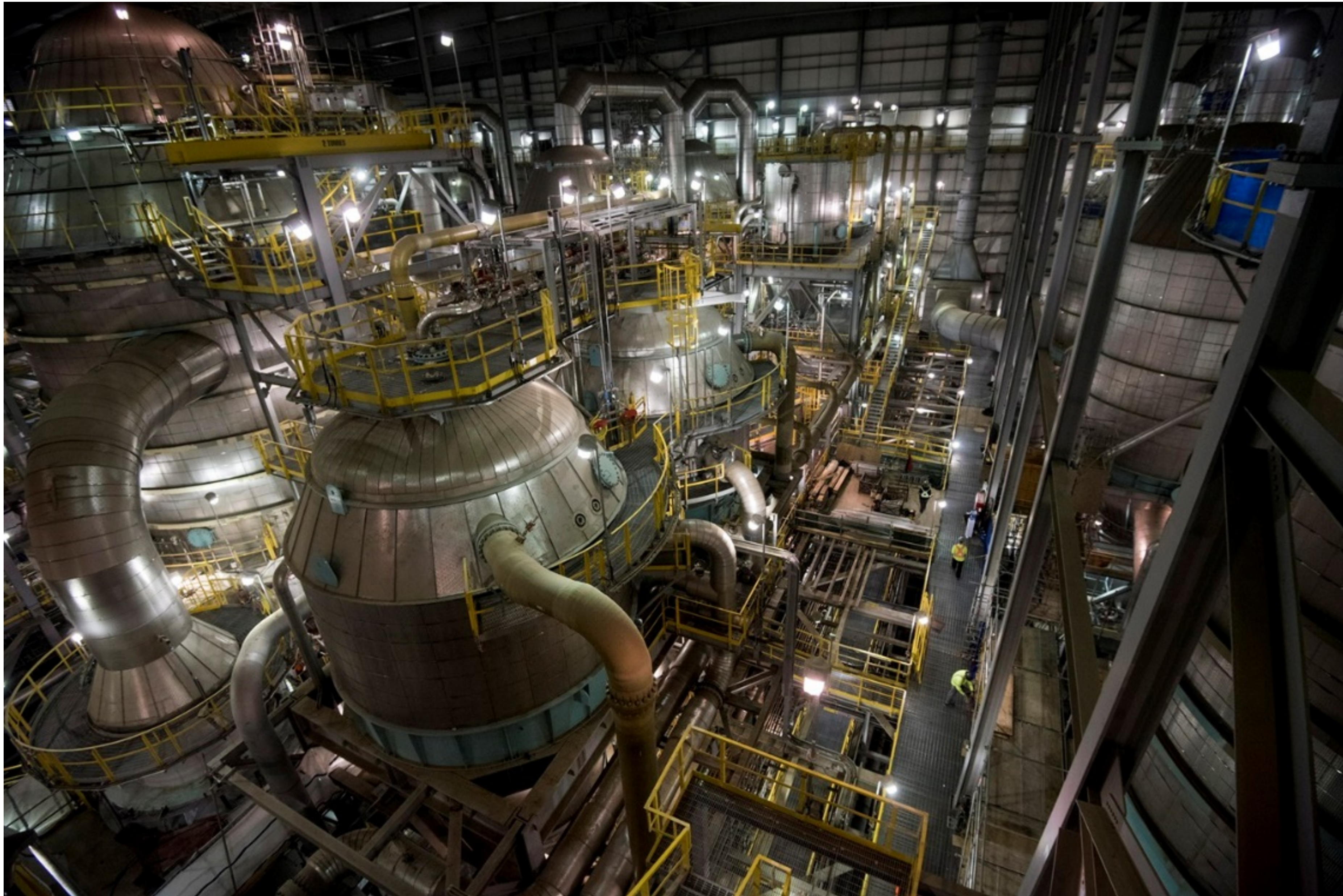
Evaporators in the wet dry area of K+S's Bethune Mine - Retrieved from https://www.680news.com/2017/05/02/ks-opens-new-potash-mine-first-new-mine-in-saskatchewan-in-more-than-40-years/
