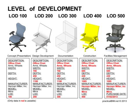
"LOD" number defines the level of completeness to which model components or elements are developed.
