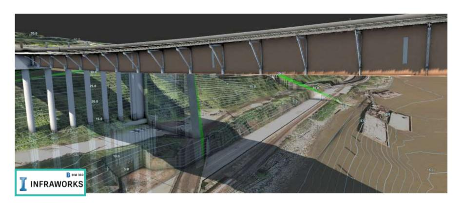
Sample Infraworks Image – Girder Splice and MUP supports
