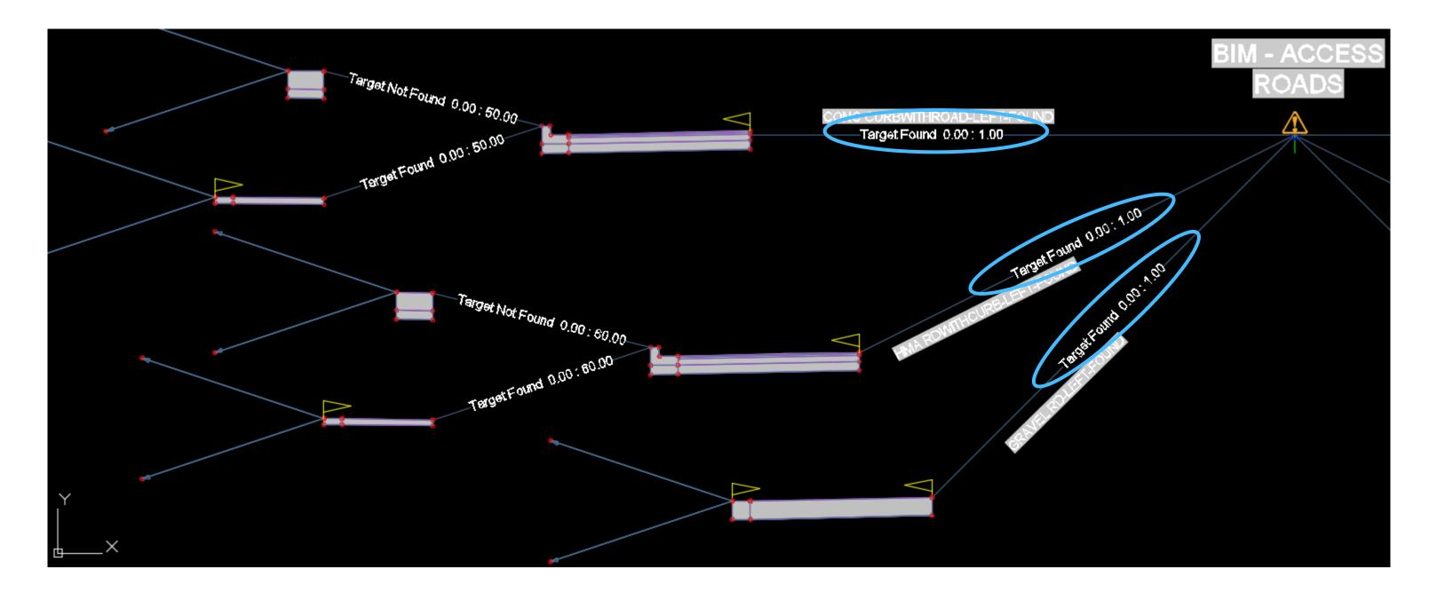
Setting the Gravel Rd-Left-Found and Gravel Rd-Right-Found conditional subassemblies, ignores the CONC, and HMA subassemblies.
