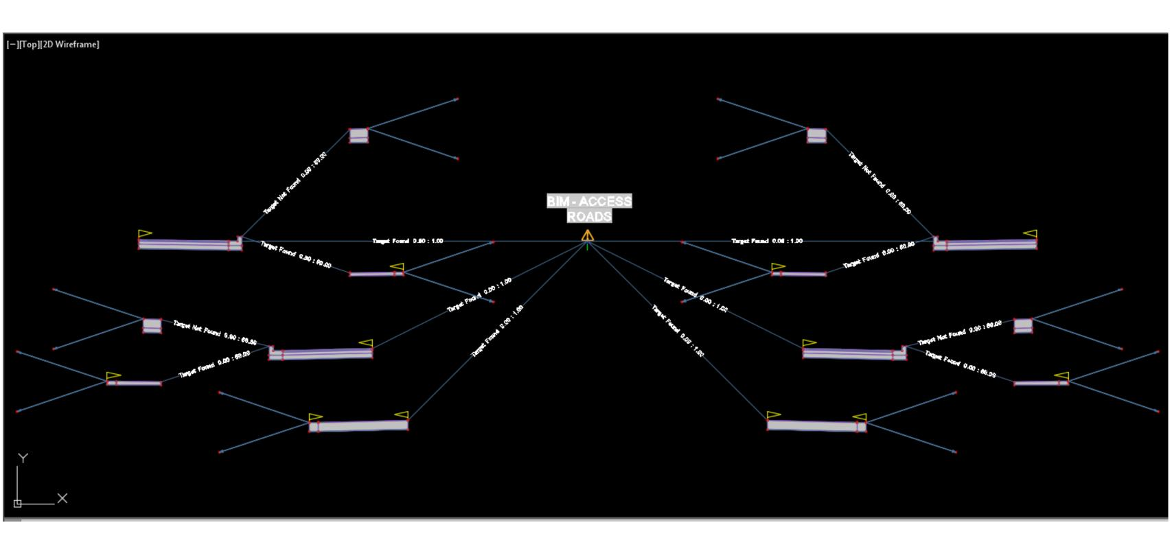
Conditional Horizontal Targets were used here to determine: Concrete, HMA, or Gravel.
