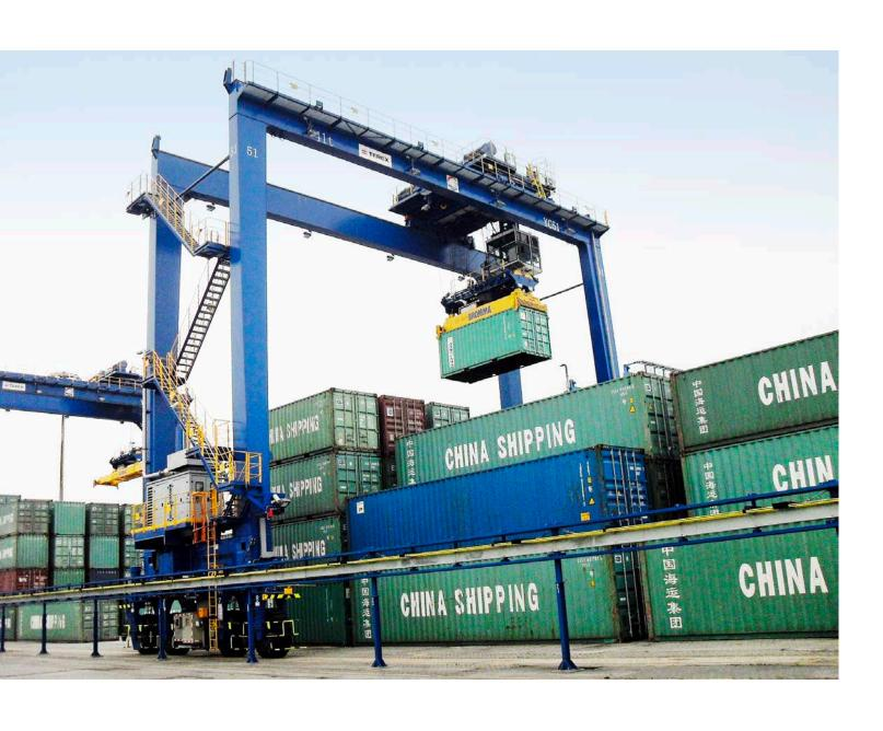
• Electrified Rubber Tire Gantry Cranes usually have the same capabilities as the standard RTGs but their drivetrain is powered by electricity rather than diesel or other fossil fuels making them the "green" alternative.
