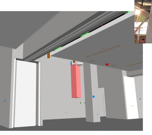
A Structural Horizontal member that spans the space or opening between two vertical supports (i.e., over a door or window)
