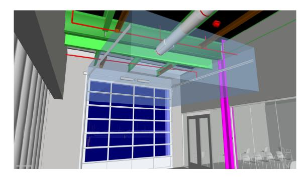
A Structural Horizontal member that spans the space or opening between two vertical supports (i.e., over a door or window).
