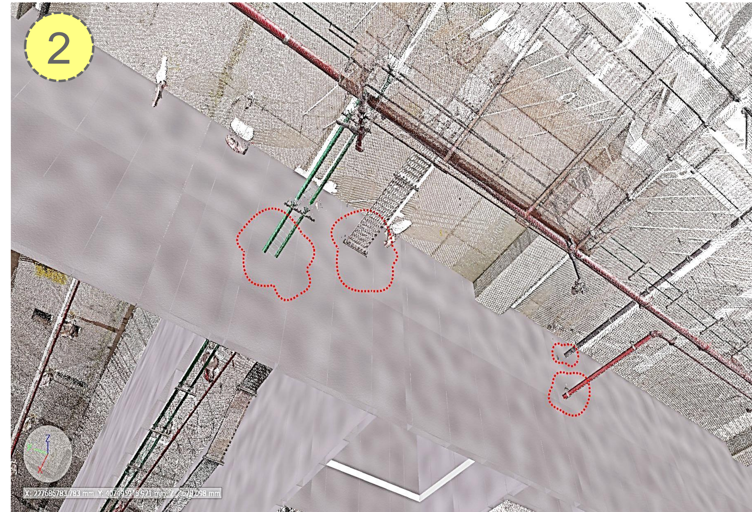
Clash between As Built Drainage, Mechanical, Fire Protection Pipe, Cable Tray and As Design AAC Panels for Cutouts
