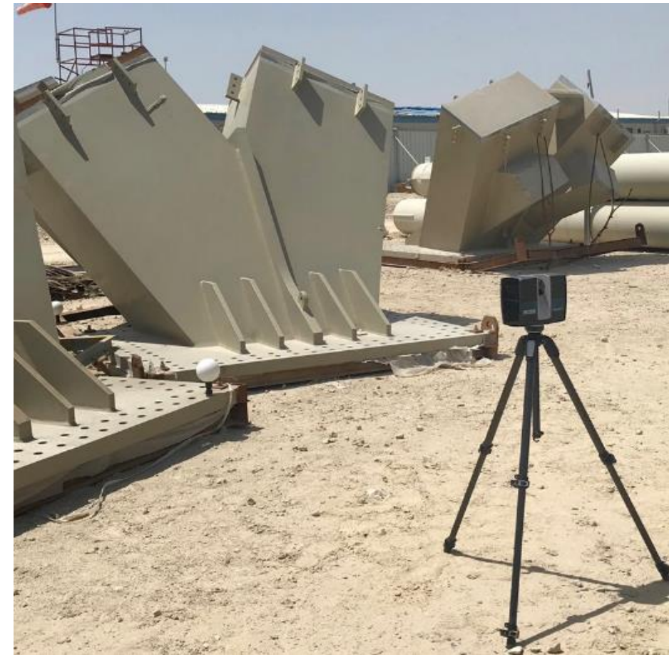
On-Site Scanning of Steel Part
