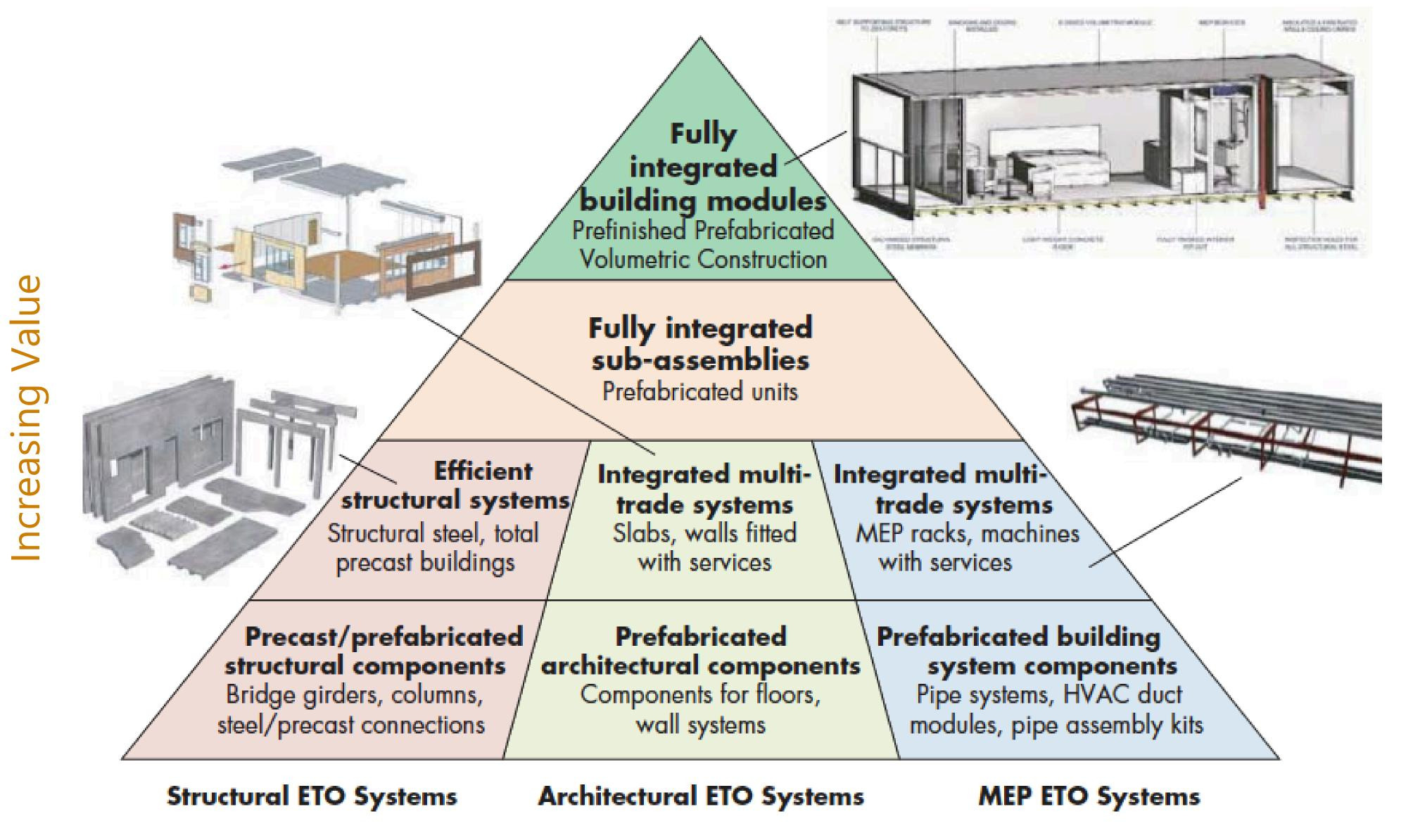
Classification of building components, according to degree of system integration and completion
