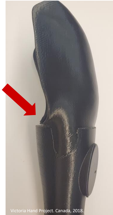
Poor Quality Socket Transition
