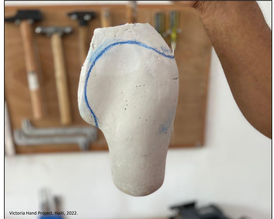
Socket Shape Sketched on Impression
