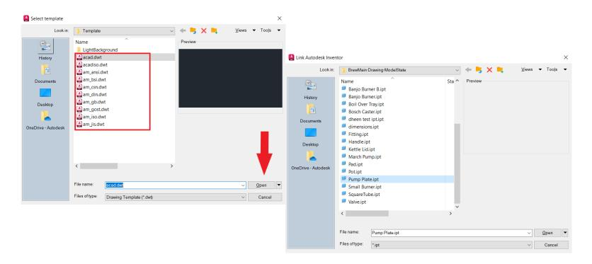
Choose the template and respective .ipt or .iam file, link is established between Inventor and AutoCAD Mechanical.
