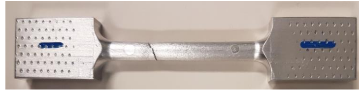
Engineering Stress vs. Strain Aluminum 2014-T651
