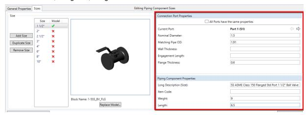
Repeat the process for the remaining valve sizes. Refer to the chart below for the remaining property values that will be used for the valves.
