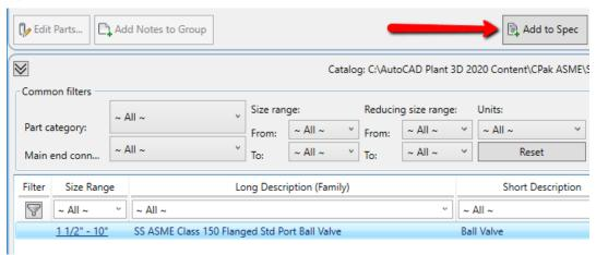
After the valve has been added to the spec, the part use priority must be set.
