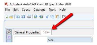
During the previous Create New Component process a size range was selected. You will now need to remove some sizes because valves were not created for all the listed sizes. Unfortunately, there is not an option to select multiple items to be removed. So, each size will need to be selected individually. From the list remove sizes 3 ½", 4 ½", 5", 7" and 9".
