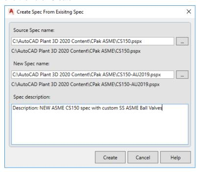
Now that you have a new spec you can add the custom valve to the spec. With the Spec Editor tab selected, you will need to browse to open the ASME Valves Catalog-AU2019.
