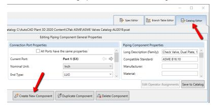
In the Create New Component window select Custom – AutoCAD DWG Block based graphics. Set the Component Category to Valves and set the Component to ValveBody. Enter the Short Description to Ball Valve, set Primary End Type to FL, set Number of Connection Ports to 2, and set Size From 1 1/2" to 10" Imperial and then click Create.
