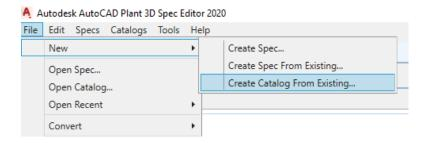
Since Spec Creator does not give you the option of creating blank Catalog, you will use the existing ASME Valves Catalog and then name the new catalog, ASME Valves Catalog-AU2019.
