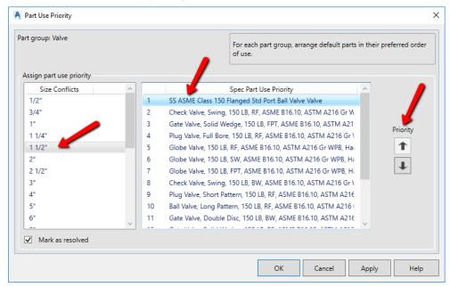
Once all the valves have been moved to the first position, then check Mark as resolve and select OK to save.
