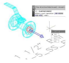
Select Accept once the other port is placed and select exit to complete the command. Repeat the process for all the remaining valve sizes.
