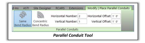
Modeling conduit in tight spaces can be difficult because Revit has a minimum bend radius that is assigned to elbows. Revit will not allow conduit to be model that has smaller bend radius that what is specified in the conduit settings. This provides real world coordination issues as you create the conduit similar to what will be seen in field when the conduit is installed.
