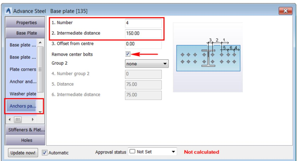
Base Plate > Anchor parallel flange tab:
