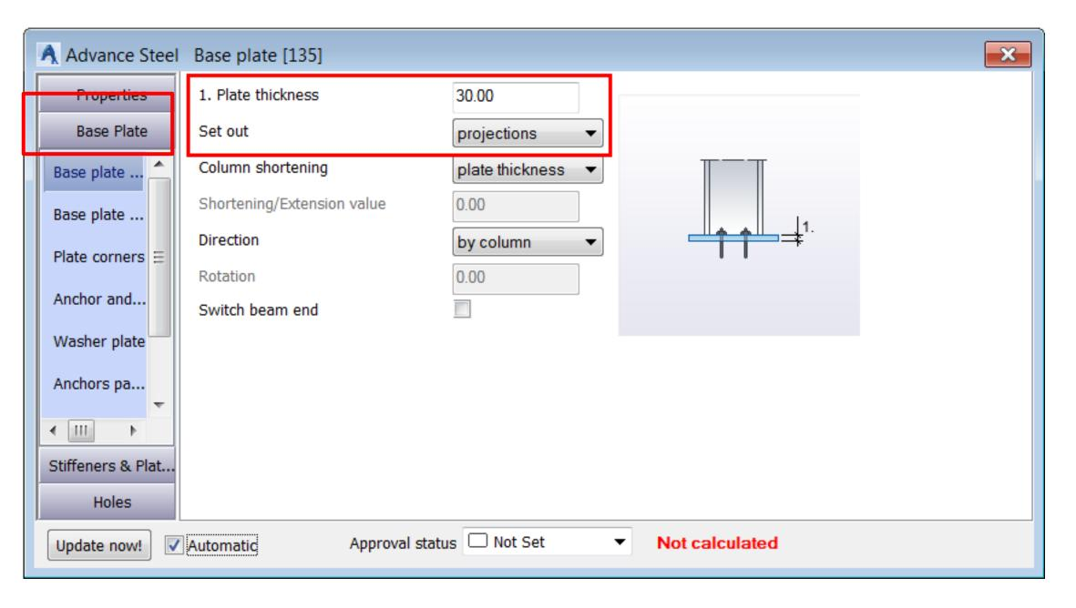
Base Plate > Base plate dimensions tab:
