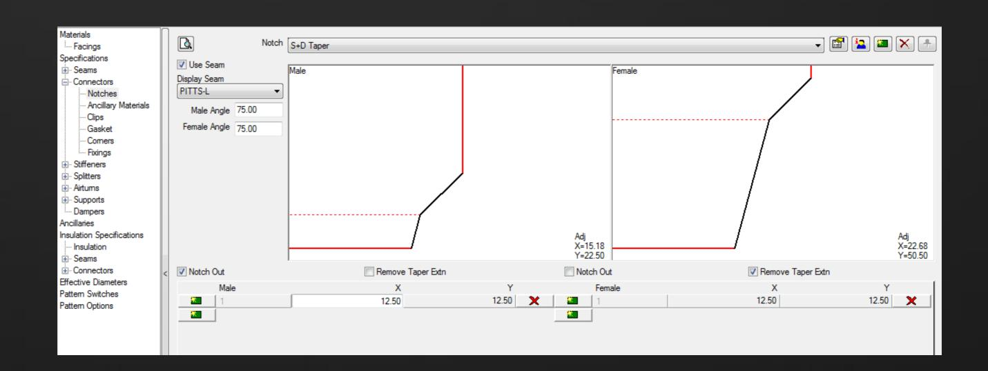
X-Y values, control length and angle of cut outs
