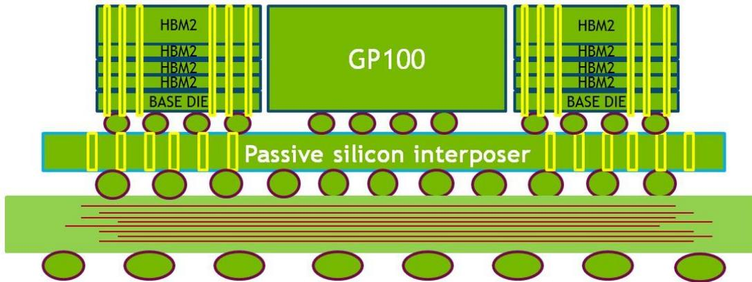
Figure 9. Cross-section illustrating GP100 adjacent HBM2 stacks
