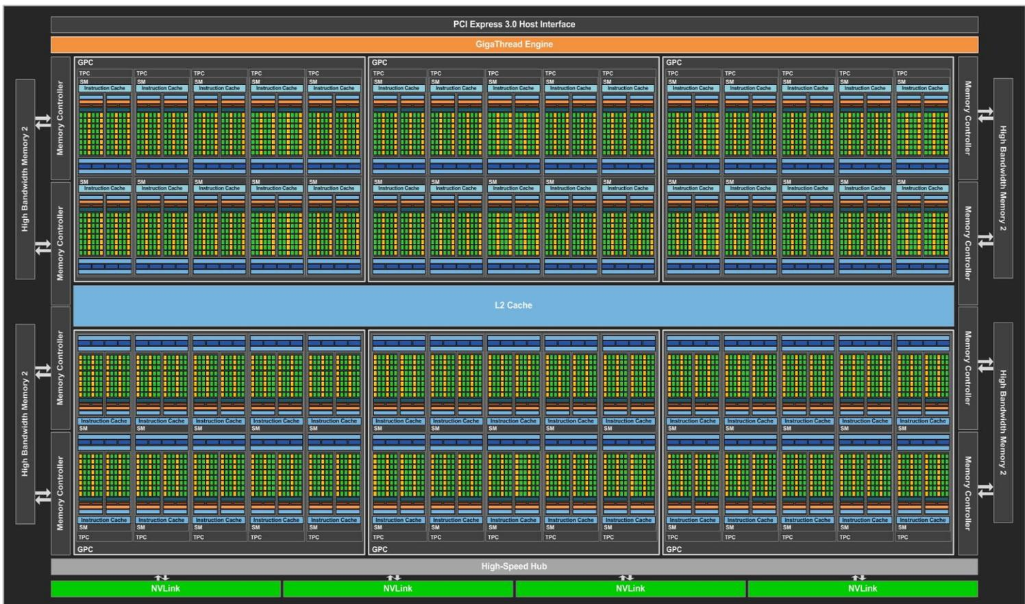
Figure 7. Pascal GP100 Full GPU with 60 SM Units
