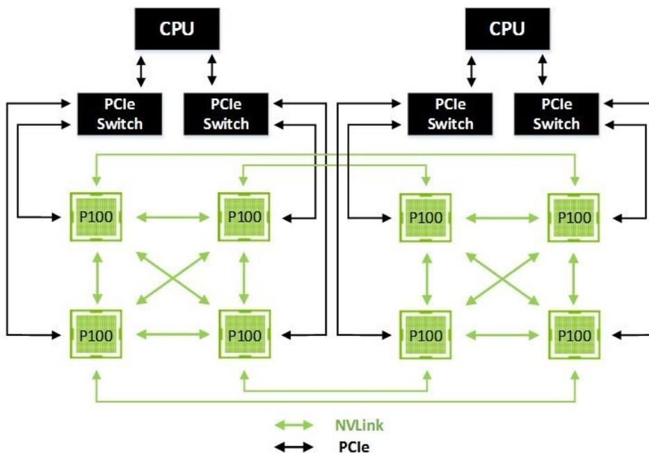
Figure 14. Eight GPU Hybrid Cube Mesh Architecture
