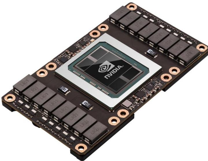
Figure 1. NVIDIA Tesla P100 with Pascal GP100 GPU
