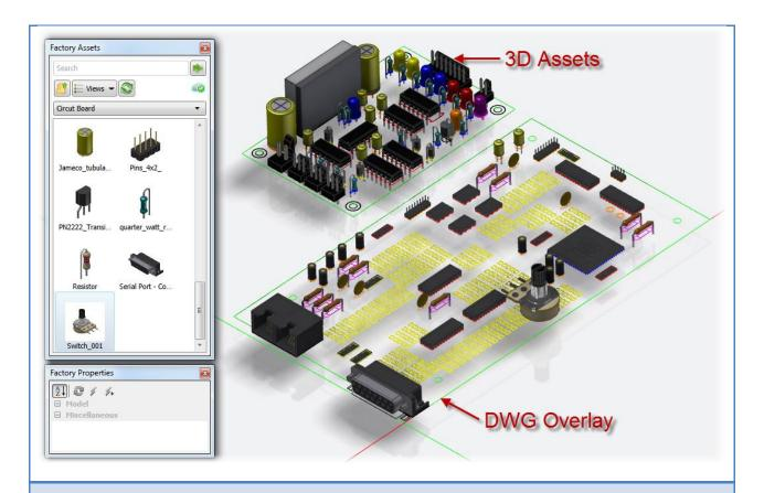
This image shows a 2D drawing of a circuit board used as the DWG Overlay. The electronic assets are placed from the Asset Browser and snapped to the 2D AutoCAD drawing.
