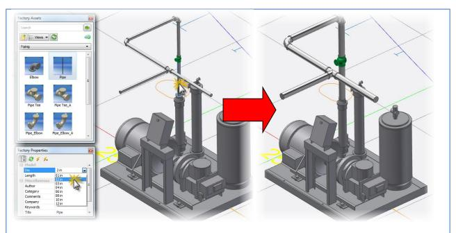
The image above shows the how easy it is to change the parameter values for a string of assets. If you change the size of one pipe, all the other pipes in the string will change as well.
