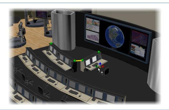
This image shows a computer desk being inserted into a command and control center. The assets placed by the Factory Design Suite automatically snap together like simple building blocks.
