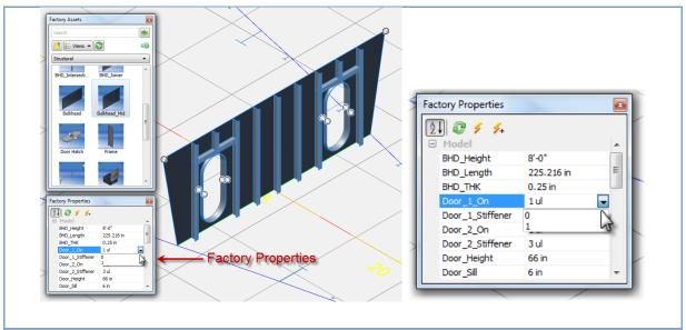
This image highlights the Factory Properties palette. The parameters of selected assets can be easily modified in this dialog.
