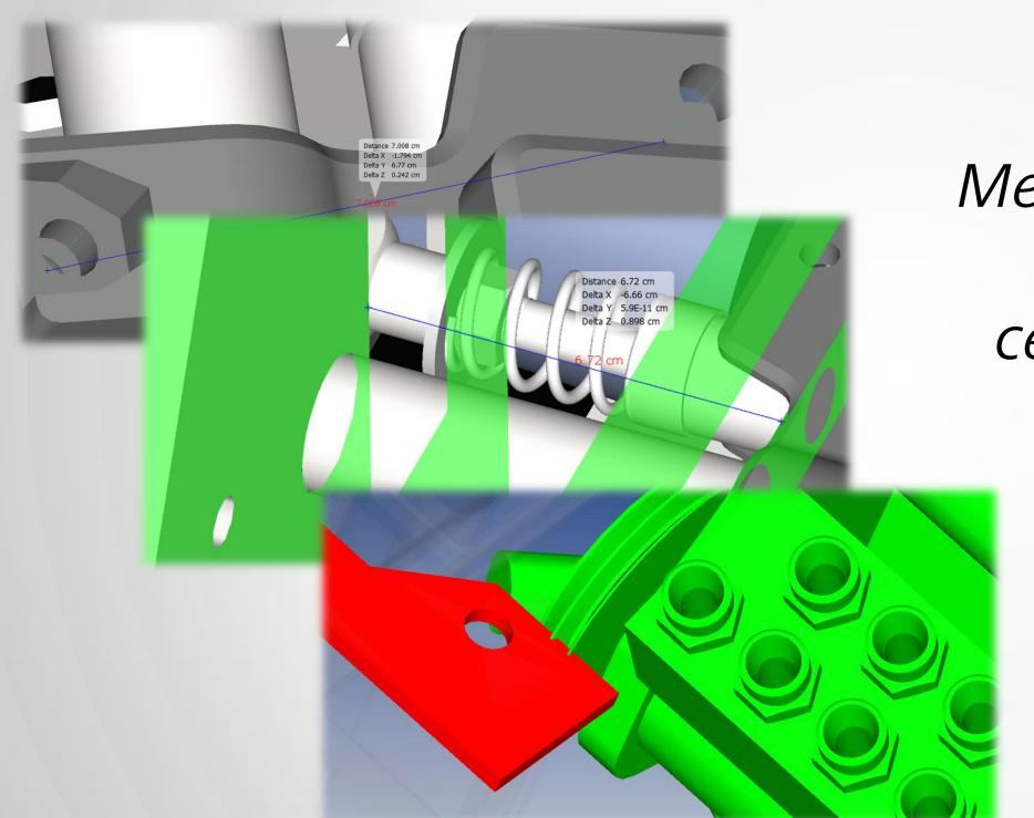
Measure minimum distances between faces, edges, centerlines, and points on mockups.
