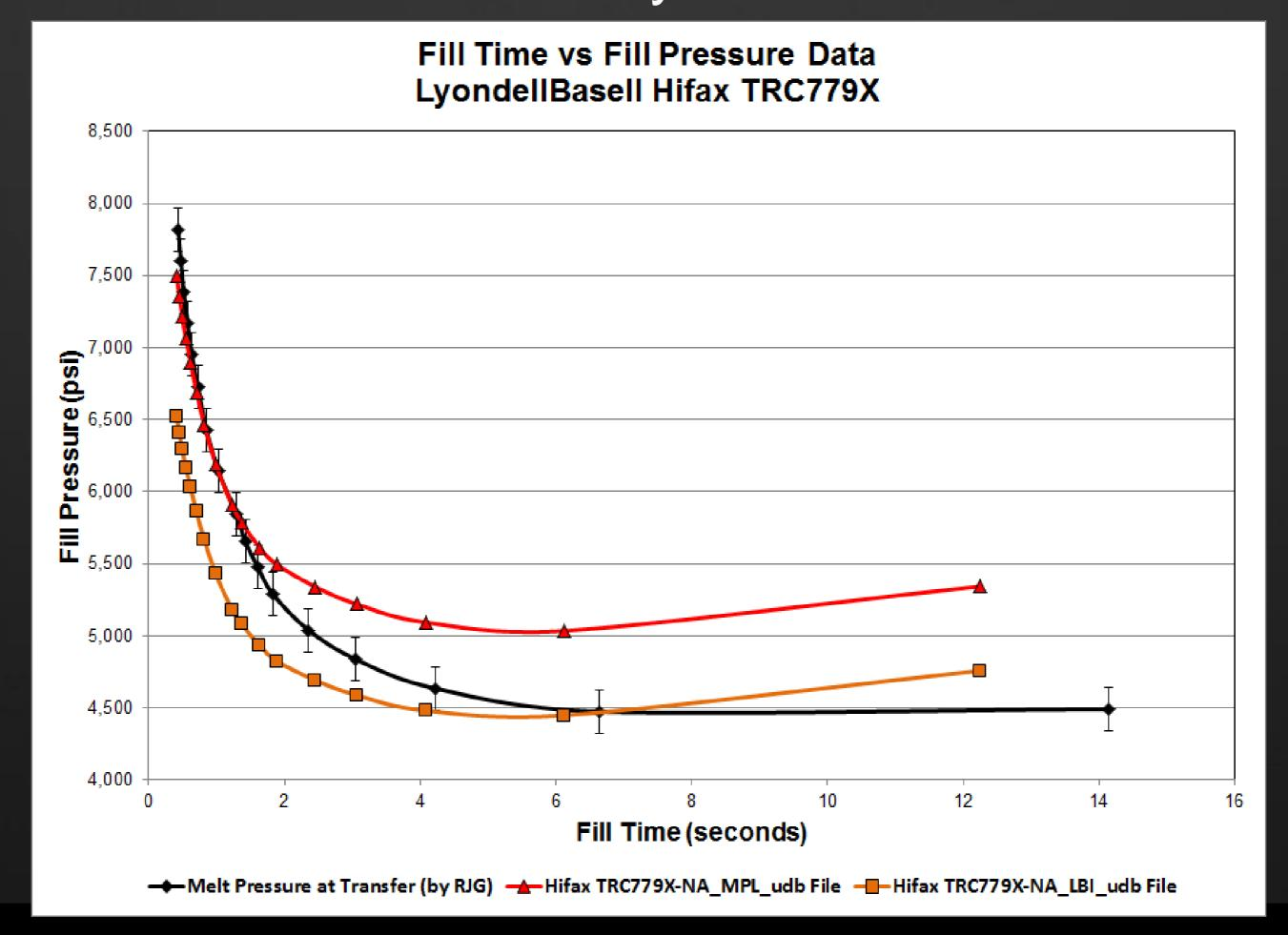
• Effect of .udb file on simulation accuracy:
