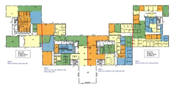
Assigning zones to the appropriate unit is a time consuming process, but must be done in order to adequately represent the HVAC system. The best way to assign zones is in the spreadsheet view of the "Air-Side HVAC" tab. In the "Basic Specifications" section, there is a dropdown menu under "Parent System" which can be changed to any of the systems currently specified.
