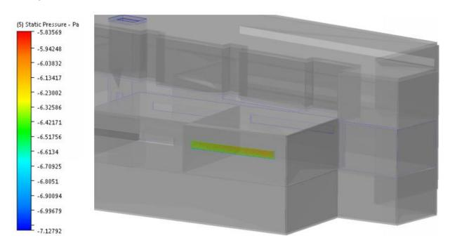
Here is an image showing the resulting static pressure on a window on the leeward side of the building:
