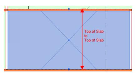
Another critical step is to use a limit offset for spaces which reside under a roof element. The offset should be at least the thickness of the roof construction element.
