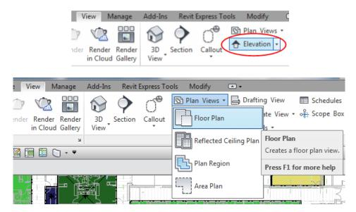
Next, create the remaining three elevations, one for each of the primary orientations. You can add additional elevations if required for specific projects.
