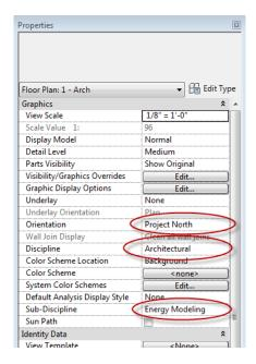
Create a view on the ground floor with the Orientation set to "True North." This will allow you to create the geometry in plan view, but be able to rotate the project True North anytime without affecting the orientation of other views. Keep the orientation set at "Project North" for all other views.
