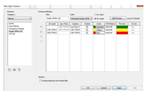
You would expect to see the highest airflows at perimeter zones (especially at the South and West) and low airflows at interior zones (especially corridors). The example below reveals this pattern.
