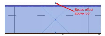
Next, use the "Place Spaces Automatically" tool that becomes available. This will create a space element in every fully bounded area. If you forget to set the space limit before placing the spaces, you can simply window select all and use the filter tool to select only the spaces. Once all spaces are selected, you can change the upper limit and offset globally for all spaces in the current view.
