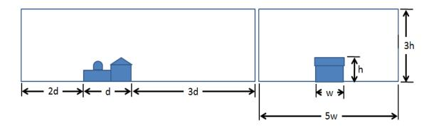
Here is an example of the analytical energy model geometry modified to include the walls, floor and roof that establish the extents of the external volume (the roof is hidden for demonstration purposes):
