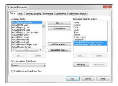
First, confirm that each space has a corresponding HVAC zone by searching the Zone column for any instances of Default. If a space is in the Default zone, that means you haven't created an exportable HVAC zone for that space. Correct this by selecting the space and clicking the Zone button under the Analyze tab.
