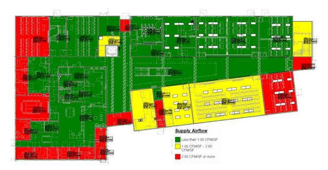
Presenting the data in this way is very powerful for QCing the load calculation and understanding the distribution of air in the building. For example, if you noticed a red zone in the core of the building, it might indicate an error with the way the load calculation was set up. Perhaps an extra zero was accidentally added to the lighting power assumption.
