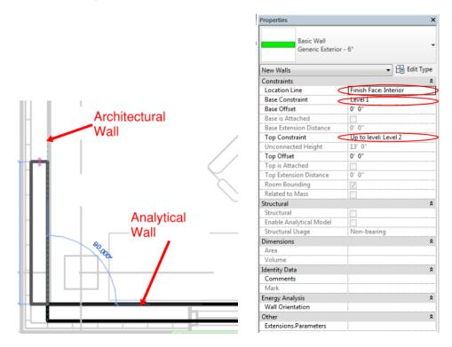
Continue tracing all the exterior walls to establish the shape of the building. Revit has several tools in the Modify tab of the ribbon that allow the geometry to be drawn much quicker than most energy modeling programs, such as trim/extend, align, array, copy, and paste.
