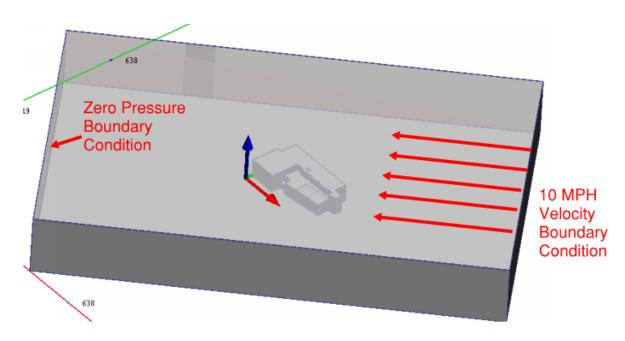
In order to simulate the average wind conditions, a velocity boundary condition is applied to the left-most surface of the external volume (the inlet). A zero pressure boundary condition is applied to the downwind surface to allow the "wind" to exit the solution field (the outlet). Notice that the building is situated off-axis from the external volume. This represents the average direction the wind blows throughout the year on this building's site.
