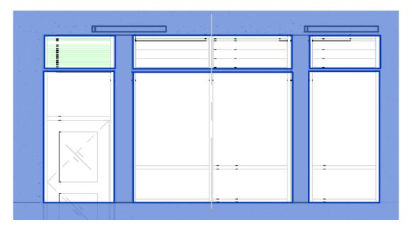
Windows can also be copied and pasted in floor plan view if the size and sill height are the same. If multiple floors have typical window arrangements, then you can use the copy and paste to selected levels tool in the same manner as with the walls. Simply lay out one of the floors and copy the typical windows up to other levels.
