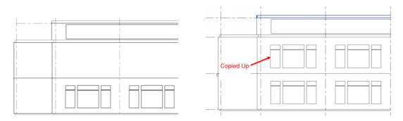
Offset the edge of the window from the edge of a bounding wall, floor, or roof by at least 0.5", even for curtain walls.
