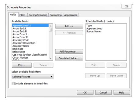
This will create a scheudle in the format shown below. This is useful for several reason. First, verify that the apparent load agrees with the luminaire schedule. Secondly, this allows you to verify that each fixture is placed in a space. If the Space:Name field is blank for any of the instances, this indicates a fixture is in the model, but not properly located in a space. Correct any issues before exporting the model.
