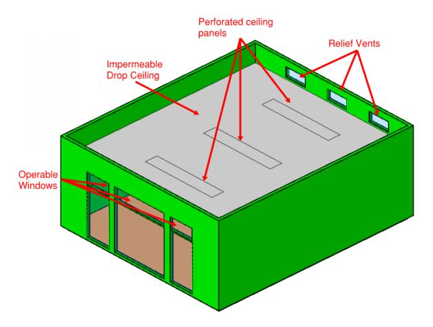
The operable windows are modeled in Revit as simple window instances. It's important to have independent windows for the non-operable windows below, so that boundary conditions can be applied only to the portion that is ventable. Similarly, four separate ceiling elements have been modeled in Revit in order to differentiate between the perforated portions and the impermeable portion. The relief vents are also modeled as simple window instances.
