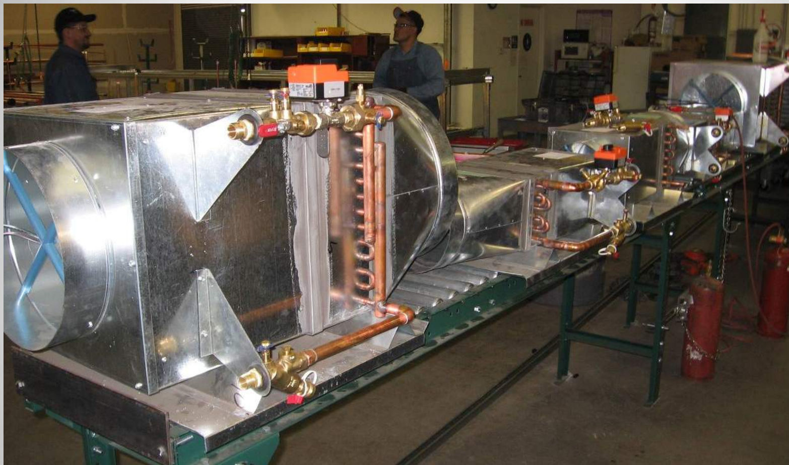
Complete VAV assembly shown. Piping, Sheet Metal and Controls are all on the assembly, tested and ready to ship.
