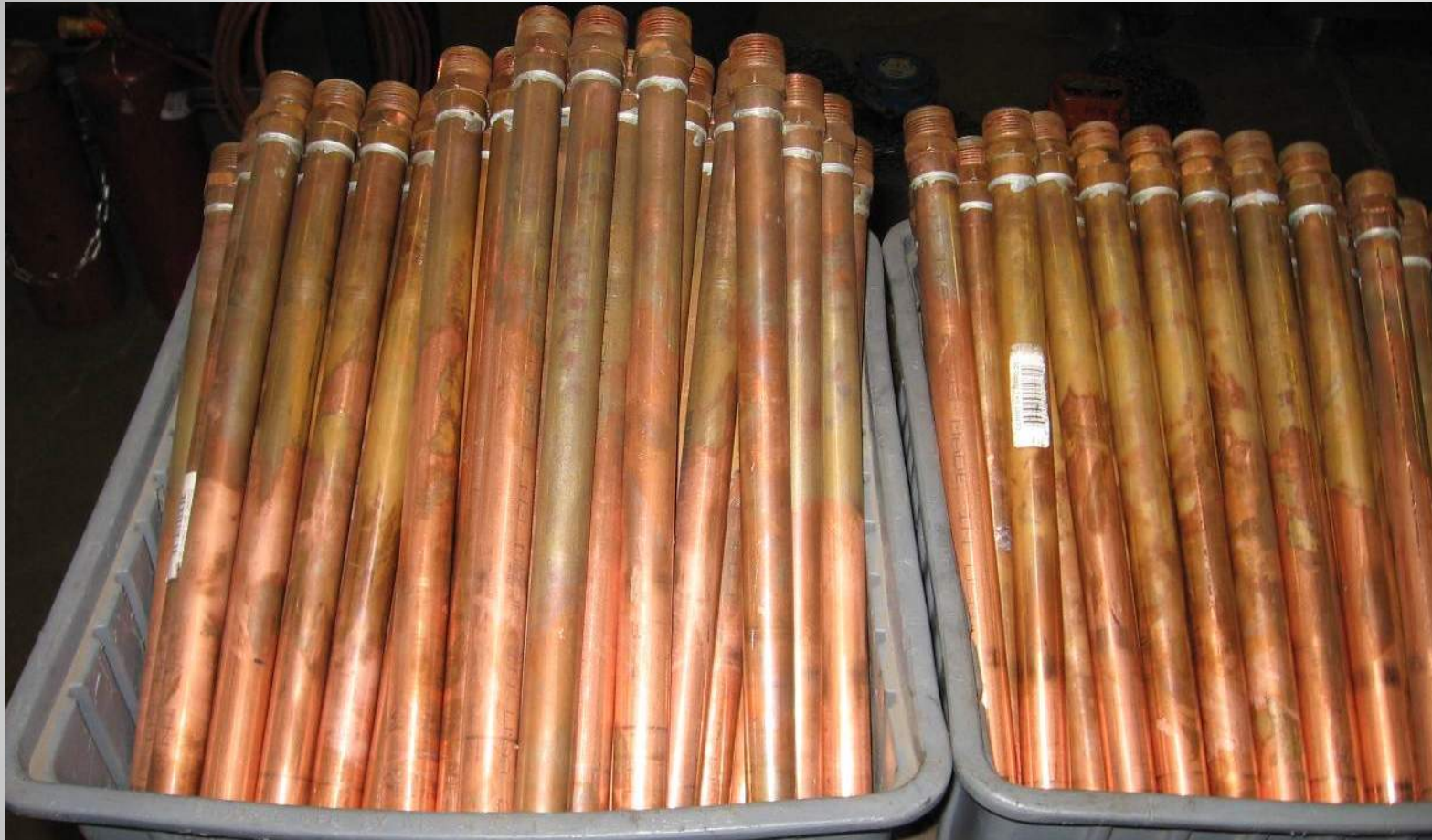
Cut copper pieces for VAV fabrication
