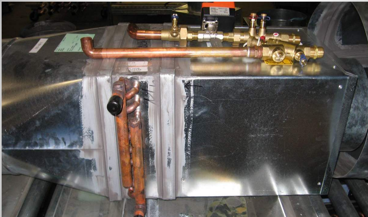
Valve and Control Kits ready to be placed on VAV
