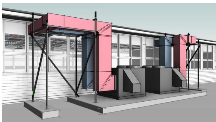
Figure 31. Seismic restraining (non-structural elements) in the model
