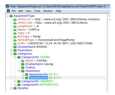
The Name property under EquipmentType should match the name of the script we create. Type can have one of three possible values: C, F, I. Type F is for fabricated equipment like tanks that uses primitives only. Type I is for converted models that use block content. Type C is for custom equipment that is completely defined by a script.
