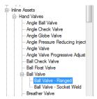
Since the Ball Valve Style is inherited from the parent Ball Valve class, we need to create a new symbol to display our flange end types. We can use the same block as the ball valve. Select the Ball Valve – Flanged class, and click Add Symbols. Use the browse button to select the projSymbolStyle.dwg for the current project. Select the PIP Ball Valve block, and set Symbol Name to Ball Valve – Flanged.
