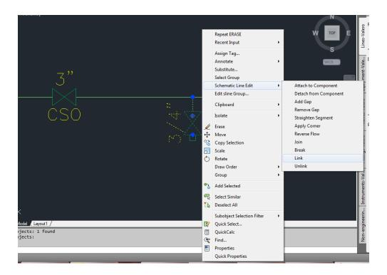
If the short pipe segment is a known, different size from its host then "add" the short segment to the host segment using the line group commands to add or remove s-lines from a group.
