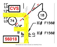
When a regulated line intersects a non-regulated line, highlight that portion of the non-regulated line that is in contact with regulated process fluid. Usually this means highlighting back to the first check valve or block valve on the non-regulated stream. See the example below in which a block valve on a steam line is highlighted because it is in VOC Vapor Service:
