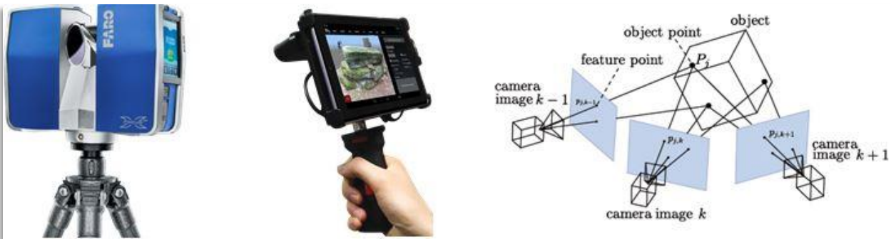
Figure 2: Capture devices from left to right: FARO Terrestrial scanner, DOTProduct multi-view photogrammetry and traditional structure from motion via digital camera
