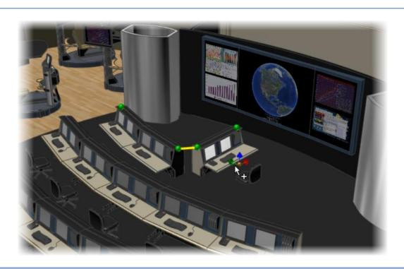
This image shows a computer desk being inserted into a command and control center. The assets placed by the Factory Design Suite automatically snap together like simple building blocks.
