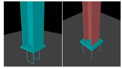
base plates are required to be oversized (anchor bolts outside of footprint and/or require a recessed pocket in the slab to avoid tripping hazard or minimize furring area requirement around the column) or if the anchors can satisfy the design loads by staying within the confines of the column footprint. Determine the pros and cons to help guide the decision. This will help the foundation detailing as it will be identified early.
